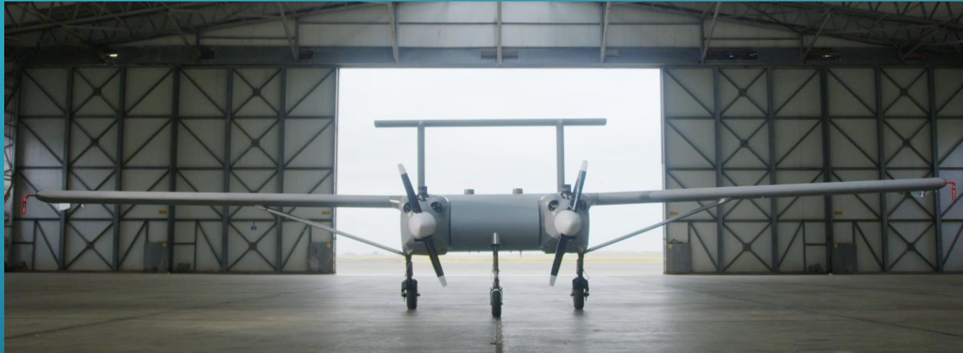
Pipistrel Cargo Drone: Nuuva V300 hybrid-electric VTOL unmanned cargo aircraft Payload: 3 Pallets – 100 CuFt and up to 3 Tonnes
